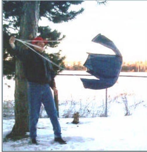
“Wind testing” of finished “1 metre” cross parachute
